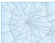
Laminated Glass TRIPLEX glass with PVB membrane
