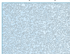
Toughened Glass Thermally Toughened glass
