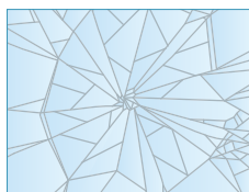
Laminated Glass TRIPLEX glass with PVB membrane
