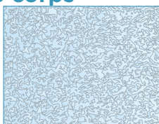
Toughened Glass Thermally Toughened glass
